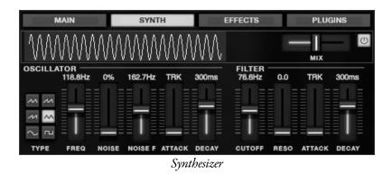
Drumagog 5 includes a more powerful synthesizer section than previous versions. Utilizing the Oscillator and Filter options, additional waveforms can be added to the drum sound, allowing a vast amount of control to enhance the resulting sound.
